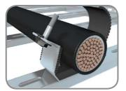
**5.** Place cable into the cleat and pull the hinged arm over the cable.
