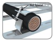
**6.** Use supplied mouth piece fittings to tighten down to no more than 8Nm using a 19mm spanner.
